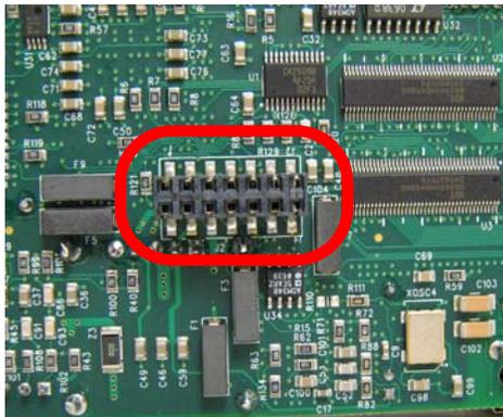
In the KP 812, the RVON-1 card connects to the KP 812 by way of the J2 connector on the RVON, attached to J37 on the KP 812 header.
