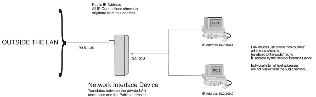
Note: A Network Interface Device can be a router, switch, gateway or anything that acts as one of these devices, such as a PC.
