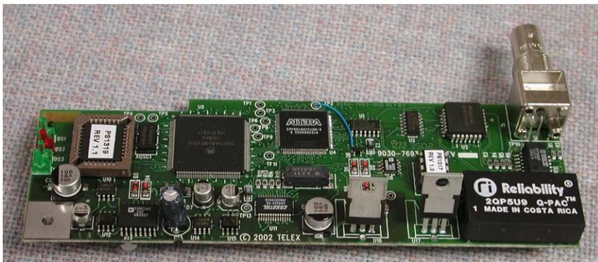
FIGURE 13. KP 832 CSI 100 Coaxial System Interface Board
